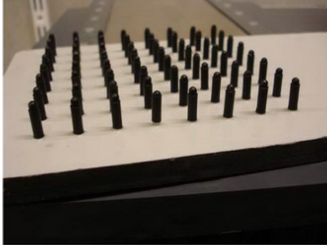
Figure 4 - Segmented anode with platinum-coated rods.
