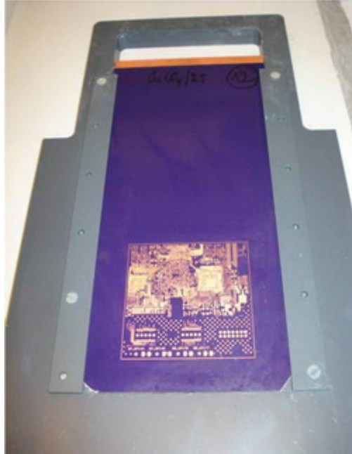
Figure 7 - Panel with Pattern 1 mounted in the cathode holder.
