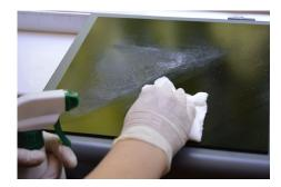
For cleaning use cold degreasing stove cleaner liquid. Use proper protecting equipment; consult the user manual or the data sheet of the material.
