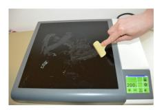
Set the device to 200°C and wait until it heats up. Remove the most remains with a metal spatula.
